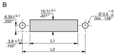
B: Panel feed-through drilling
