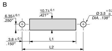
B: Panel feed-through drilling
